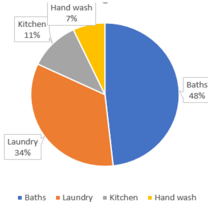
Figure 1.2: Greywater distribution of house in L/day (New South Wales Population Health Survey 2006 (HOIST))
